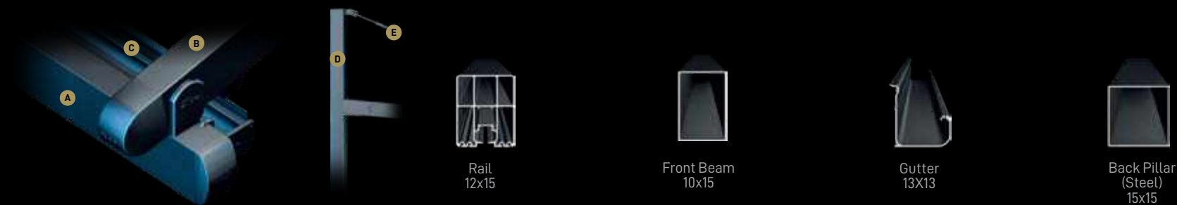
A Front Beam B Rail C Gutter D Back Pillar E Hanging Pipe (Ø 50)
